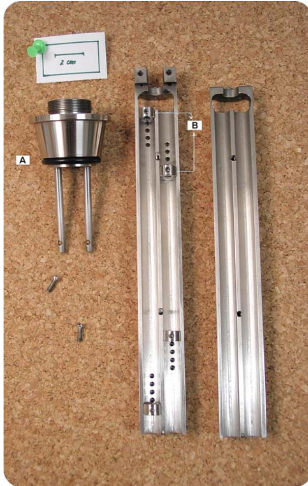
Fig. 1. Stainless steel measuring cells. A – cell top and also part of the sealing vessel cap. B – Soldering end supports for the wires: a stainless steel hook, tungsten tape, and small tungsten weight comprise the fixation mechanism.
